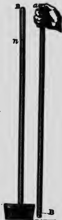
FIG. 127. — The barometer tube and mercury. In the complete instrument a scale of inches stands beside the tube, the zero of the scale being at the level of the mercury surface outside the tube.
